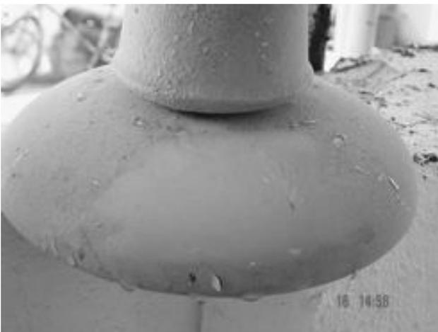
**Figure 12:** Hydrophobicity measurement on an RTV SIR coated porcelain insulator. The contamination layer has been removed and a hydrophilic behaviour is observed.
