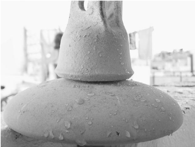
**Figure 11:** Hydrophobicity measurement on an RTV SIR coated porcelain insulator with a contamination layer.
