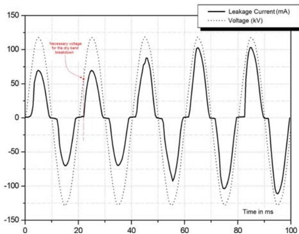
Figure 15 Influence of the dry band to the LC waveform in the case of porcelain insulators
