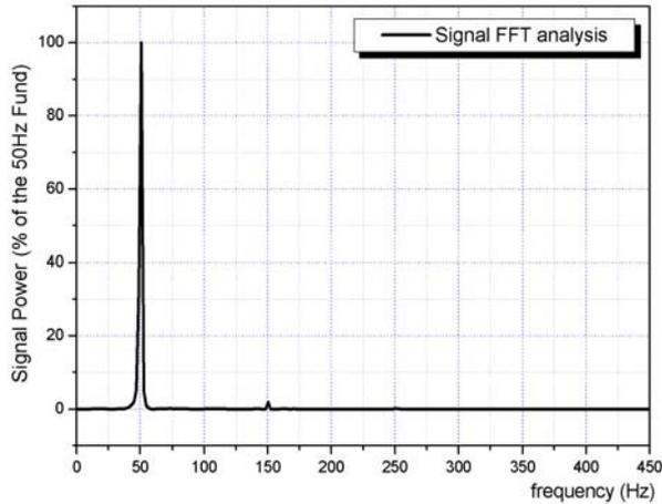
Figure 5 FFT Analysis of the LC in fig. 4
