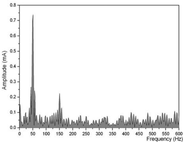
Figure 11 FFT Analysis of the LC in fig. 10
