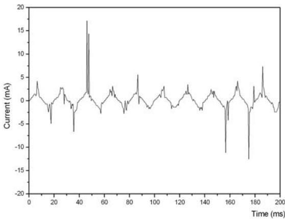
Figure 10 LC during dry band activity and water droplets corona in the case of SIR Insulators
