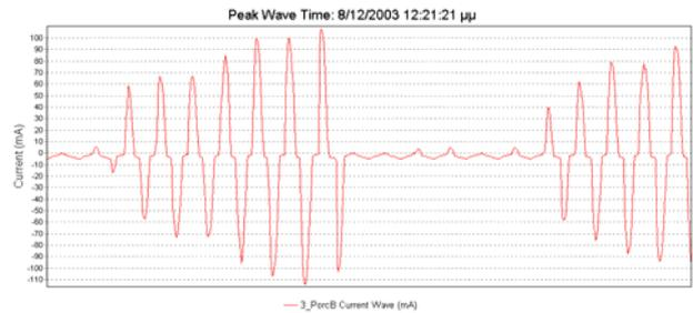
Figure 7 LC during dry band activity
