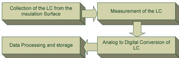
Figure 2 The four stages process in the measurement of LC
