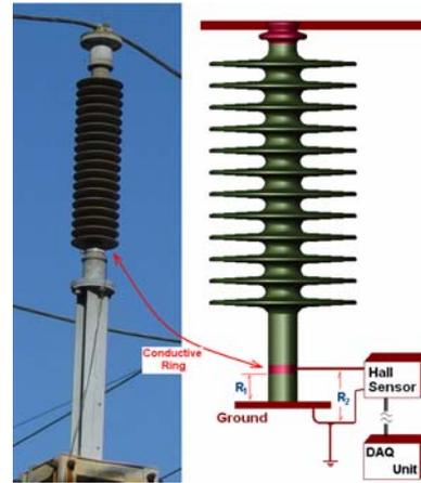
Figure 3 The measurement setup
