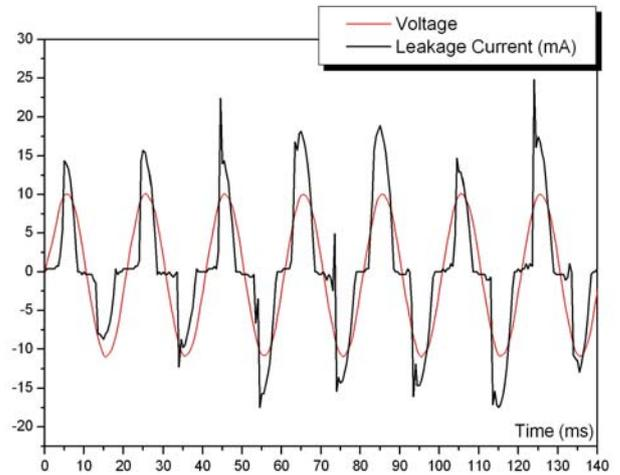
Figure 12 LC during dry band activity in the case of SIR Insulators
