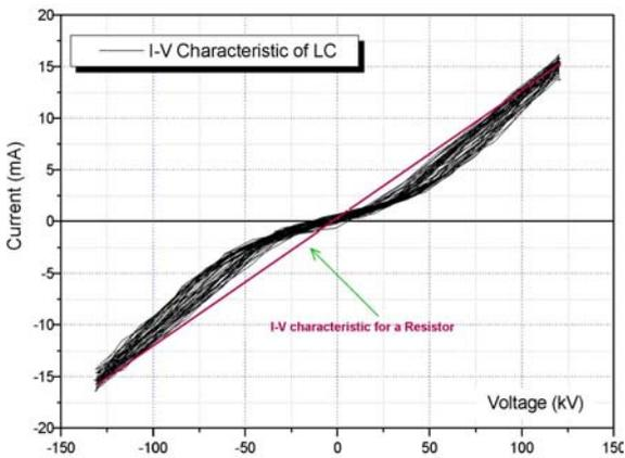
Figure 6 I-V Characteristic for the LC in figure 4
