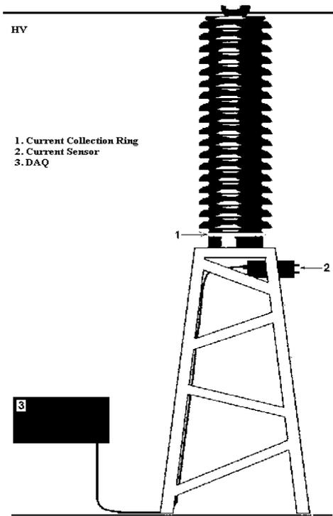
Figure 1. A schematic representation of the LC measuring apparatus
