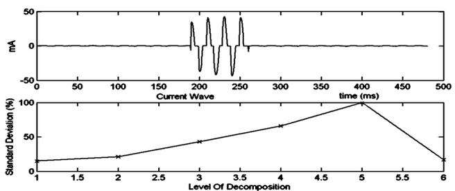
Figure 4. A Type B waveform and the STD\_MRA pattern
