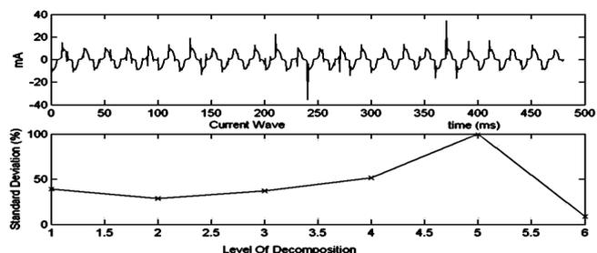
Figure 5. A Type C waveform and the STD\_MRA pattern
