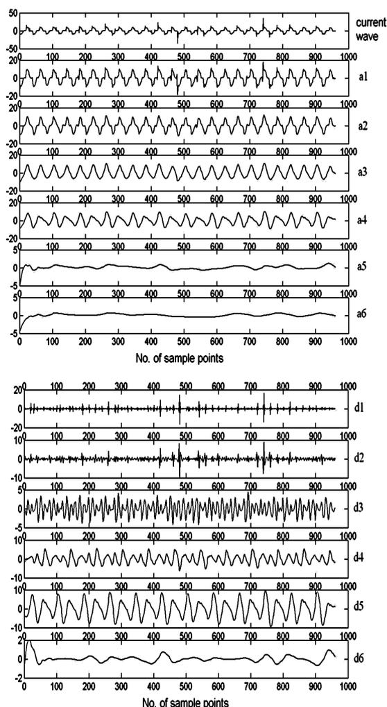
Figure 2. Six level MRA analysis of a LC waveform. a1-a6 shows the approximation and d1-d6 shows the details through levels 1-6.
