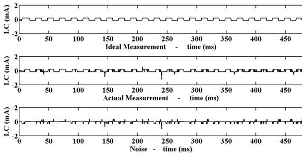
**Figure 5:** A LC measurement of low amplitude. The ideal (noise-free) measurement, the actual measurement and the extracted noise.
