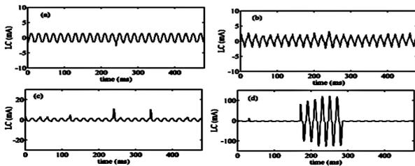
**Figure 2:** Field Measurements: Typical waveform shapes: a) sinusoid b) distorted sinusoid c) pulses superimposed at the waveform crest d) dry band arcing
