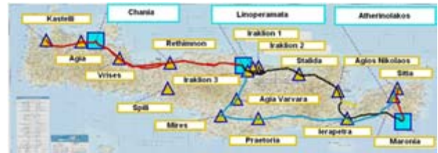
Fig. 1. The power system of Crete. Squares denote step-up substation/power plants and triangles denote step-down substation
