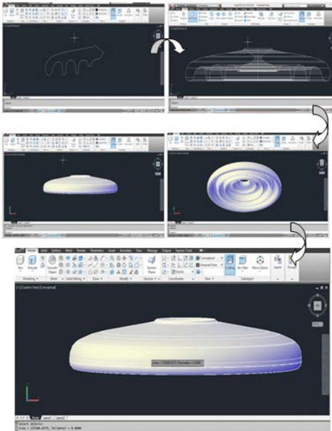
Fig. 7. Calculating an insulator’s surface area using Autocad
