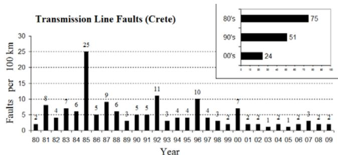
Fig. 4. Transmission Line faults (1980-2010) per 100 km
