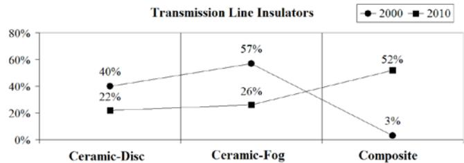
Fig. 3. Transmission line insulator percentage from 2000 to 2010
