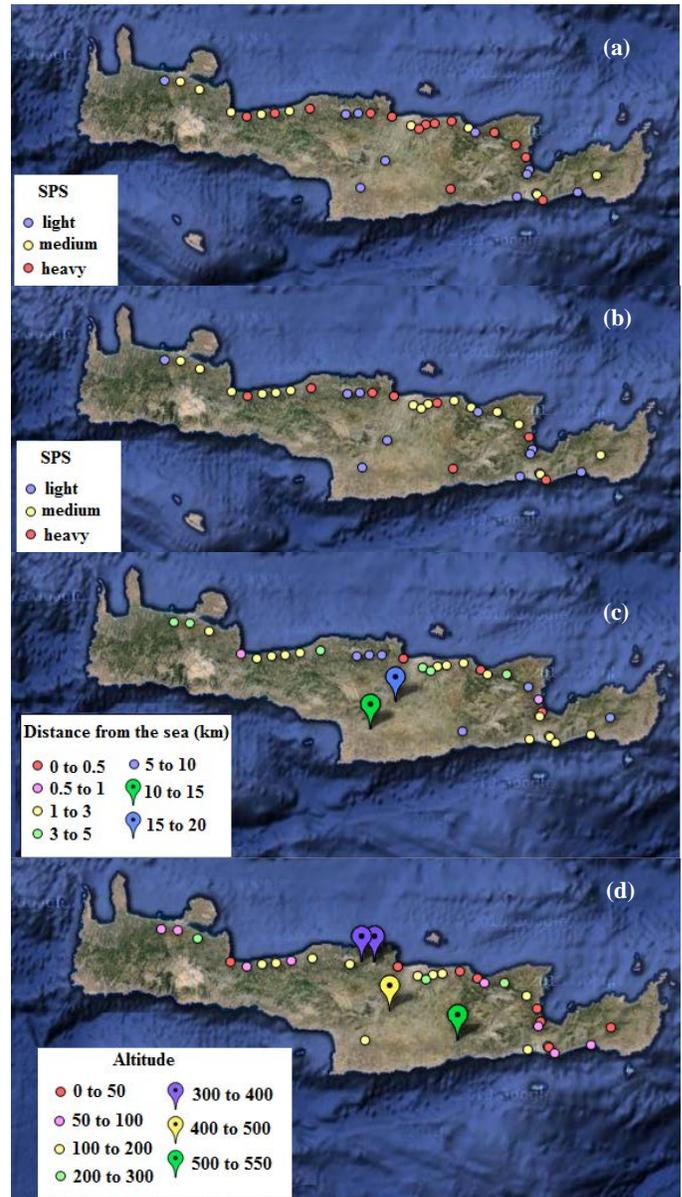
Fig 8. (a) SPS classes according to IEEE (b) SPS classes according to CIGRE (c) the minimum distance from the sea for each tower (d) the altitude of each tower
