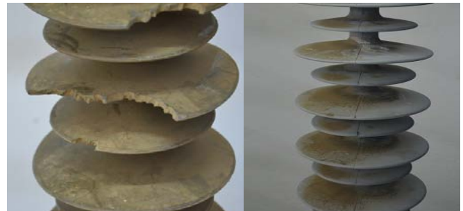
Fig. 2: Fault insulators in high voltage power system of Crete
