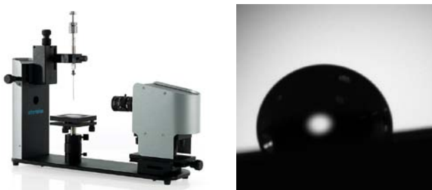
Fig. 10: Contact angle device (left) and measurement (right)
