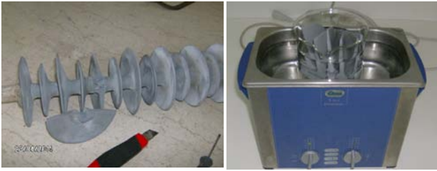
Sampling from a field high voltage composite insulator; 150 kV network of Crete
