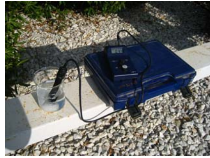
Fig. 2. Measuring ESDD on site
