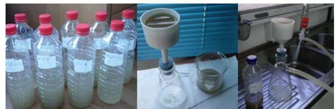
Fig. 4. Labelled bottles with solutions, filtering and filtering assisted with a water vacuum pump
