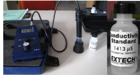
Fig. 3. Calibration and accuracy verification using a solution of standard conductivity
