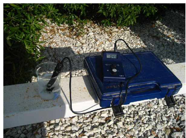
Fig. 6 Measuring ESDD on site
