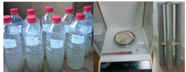
Figure 10. Labeled bottled with the remaining solution after ESDD measurements, the precision scale in HEDNO's chemistry lab weighing a dried filter, and the result of a first attempt to fabricate a DDDG measuring kit
