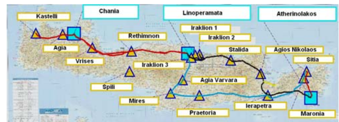
Figure 1. The power system of Crete. Squares denote step-up substation/power plants and triangles denote step-down substation.
