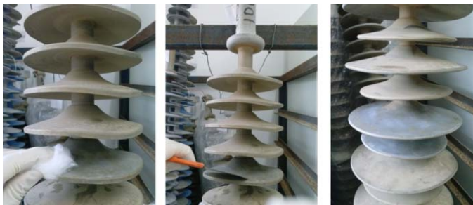
Fig. 8. ESDD measurement on a HTV-SIR insulator removed from the network
