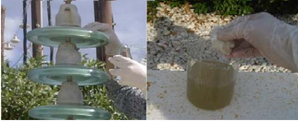
Fig. 1. Measuring ESDD on site
