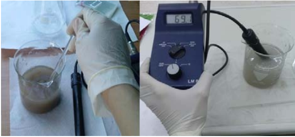
Fig. 2. Measuring the conductivity of the solution
