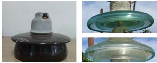
Fig. 7. 150 kV specimen insulators
