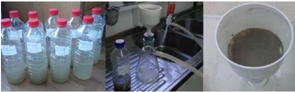
Fig. 3. Solutions into labeled bottles, filtering with water vacuum pump and residuum on the filter paper
