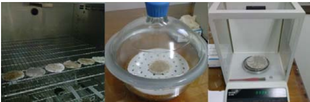
Fig. 4. Filters in the drying oven, desiccator and precision scale
