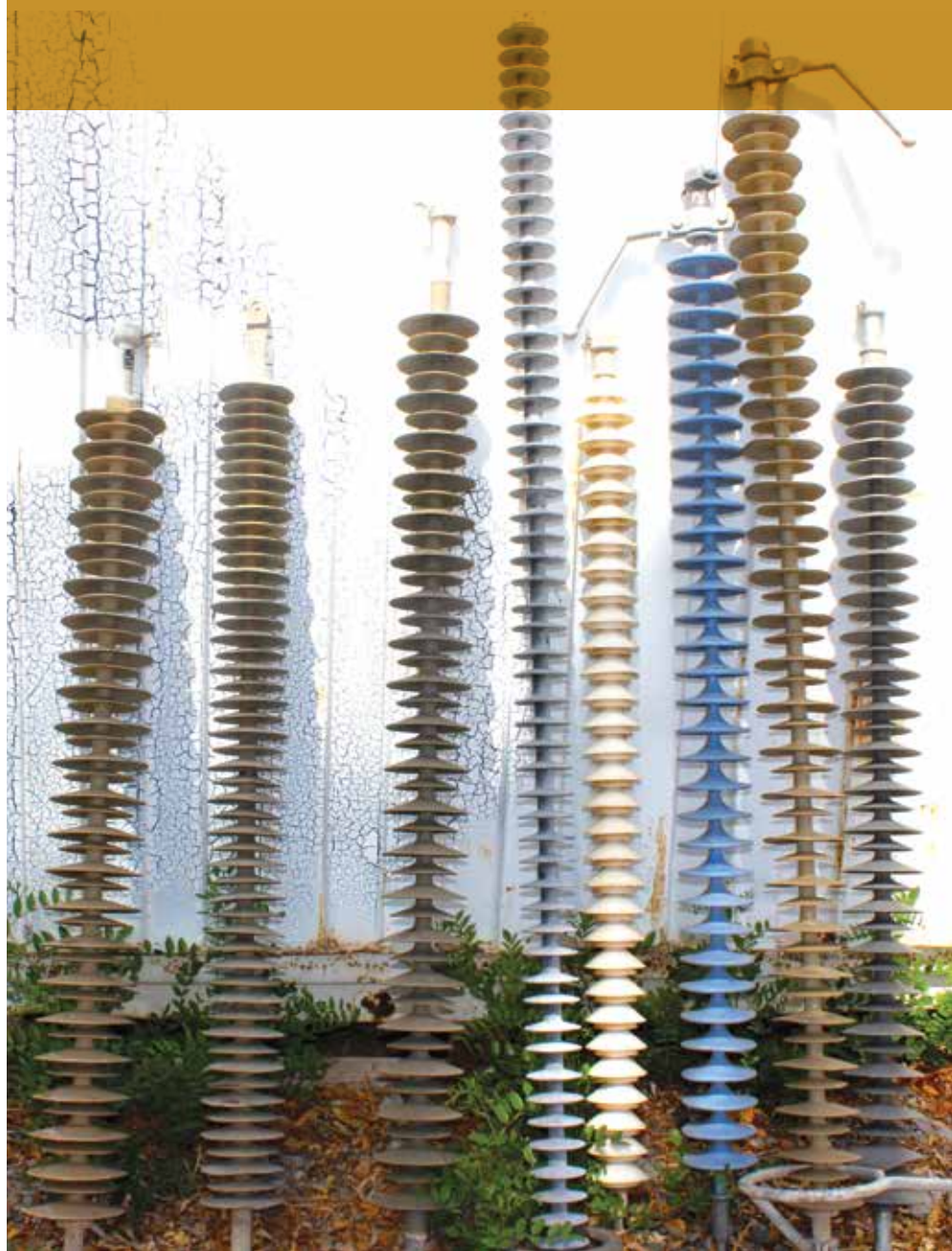
Selection of 150 kV composite insulators removed from service.
