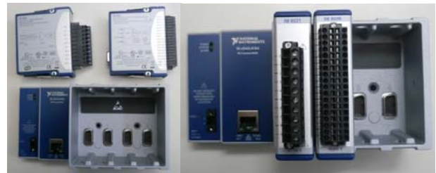
Fig. 4. NI Compact DAQ 9184 chassis equipped with a NI 9221 and a NI 9205 module
