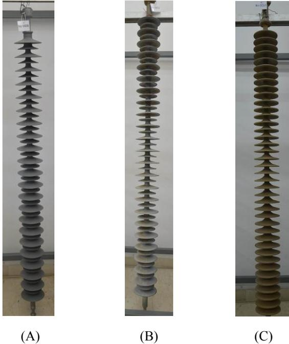
Fig 3 (a): Composite Insulators; (A) new, (B) field aged EPDM, (C) field aged SIR.
