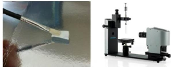
Fig 4: Deposition of slurry on samples surfaces (left), Contact angle instrument KSV-CAM 101(right).
