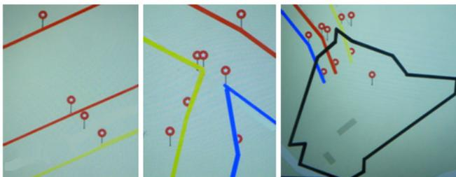
Fig. 7. Multiple placemark representation with the line axes deselected for viewing. Left: a single circuit line (up) and a double circuit line (down). Middle: the "junction" depicted in the lower left image of Figure 3. Right: entering a substation (an extra placemark is used for the substation and the area limits are drawn in black) (screenshots from Mapswithme/Maps.ME version 4.4.3, Map data from OpenStreetMap)
