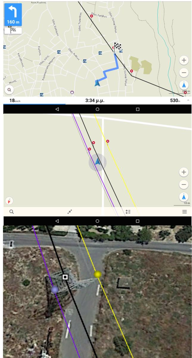
Fig. 11. Upper image: navigating to a certain tower (only tower and axes shown). Middle image: reaching the tower (turning on all placemarks). (Screenshots from Mapswithme/Maps.ME version 6.5.2, Map data from OpenStreetMap). Lower image: View of the tower in Google Earth Pro (Screenshot for Google Earth Pro, Map data: Google).
