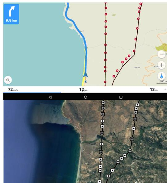
Fig. 9. Upper image: Navigation with tower and axes placemarks on (Screenshot from Mapswithme/Maps.ME version 6.5.2, Map data from OpenStreetMap). Lower image: The same area as shown in Google Earth Pro (Screenshot from Google Earth Pro, Map data: Data SIO, NOAA, U.S. Navy, NGA, GEBCO)
