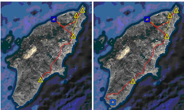
Fig. 1. The power system of Rhodes. Left: current scheme, Right: near future scheme. Squares denote power plants and triangles denote step down substations. Red line denotes a double circuit and yellow line denotes a single circuit. (Screenshots from Google Earth Pro, Map data: Google, Image LandSat, Data SIO, NOAA, U.S. Navy, NGA, GEBCO)
