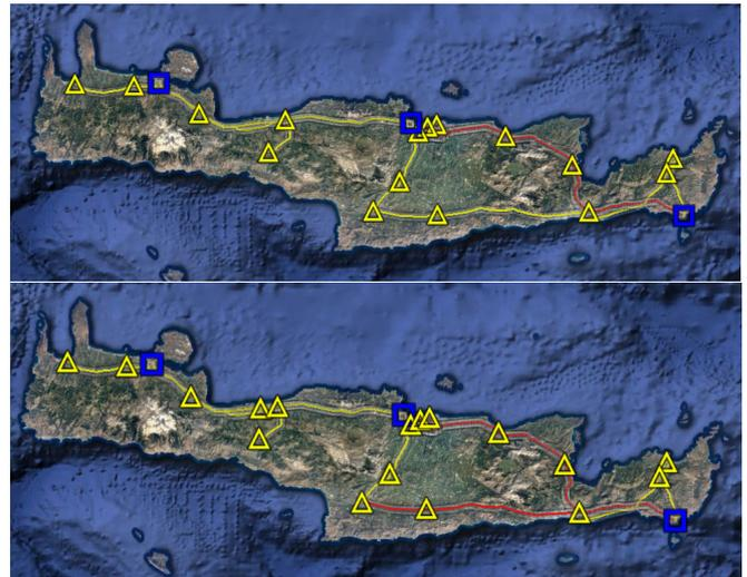
Fig. 2. The power system of Crete in 2016. Up: current scheme, Down: near future scheme. Squares denote power plants and triangles denote step down substations. Red line denotes a double circuit and yellow line denotes a single circuit. (Screenshots from Google Earth Pro, Map data: Google, Image LandSat, Data SIO, NOAA, U.S. Navy, NGA, GEBCO)
